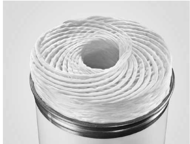
Fig.5 Precise coiling of Polyester slivers thanks to CLEANcoil-PES coiler.
