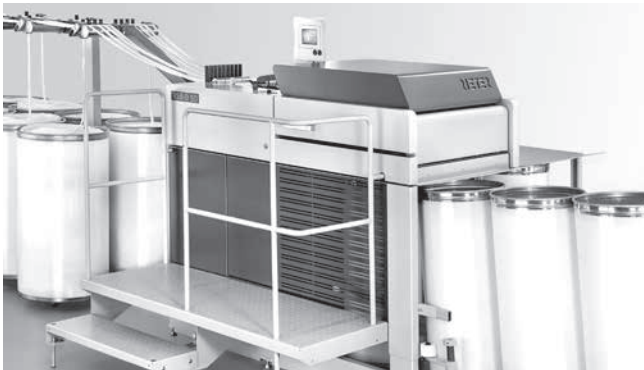
Fig. 1 RSB-D 50 draw frame highest productivity with 1 200 m/min delivery speed.
